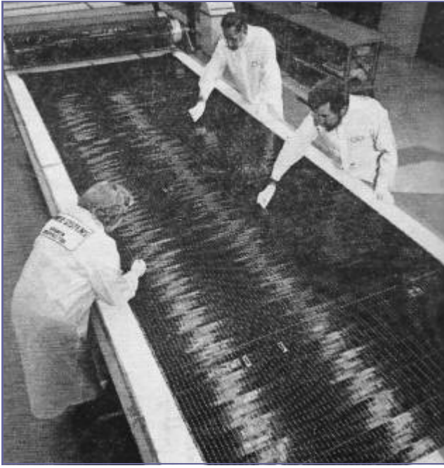
Fig. 8 - Panel of solar cells for a Hughes FRUSA (Flexible Rolled-up Solar Array).
