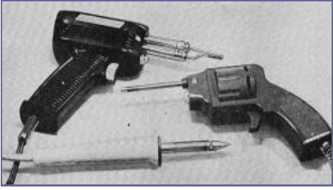
Clockwise from bottom, pencil soldering iron, transformer soldering gun, and soldering pistol are most often used types of soldering tools. Each type of tool is available with different heat power ratings plus a variety of specialized tip configurations.
