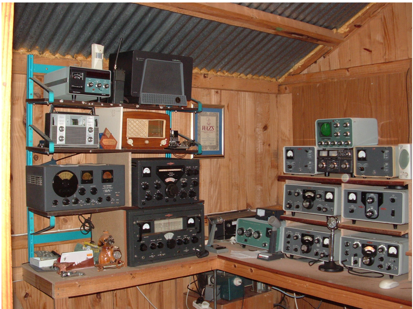
The first of the Collins equipment : 75A-4 Rx; 32V-3 Tx; SB200 Linear; 32S-3 Tx; 75S3 Rx; Station Control x 2; Heathkit SB620 Scope; 30L-1 Linear; KWM2-A Transceiver and an FC102 Ant tuner in between.
