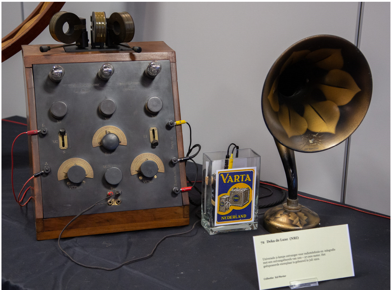
Beautiful handcrafted and machined Idzerda 3-valve receiver 1920/21; Courtesy by Piet Blaas NVHR
