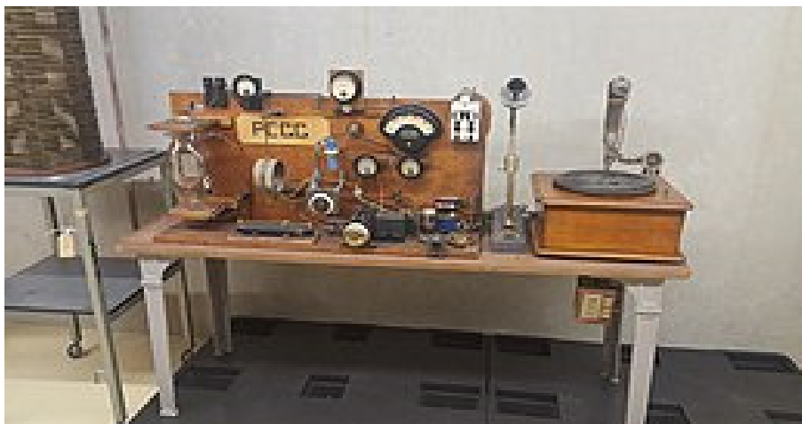
A replica of Idzerda's first transmitter 1919. In the horn speaker arm of the "Pathfoon" is a carbon mic. The transmitting triode as well as a huge antenna loading coil is on the left hand side (on the trolley table).
