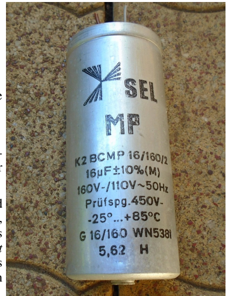
Picture 1 Metallised paper foil non-polarised capacitor. Date code is May 1962
