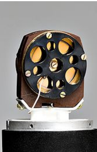
Inside the Oktava 319 condenser microphone
