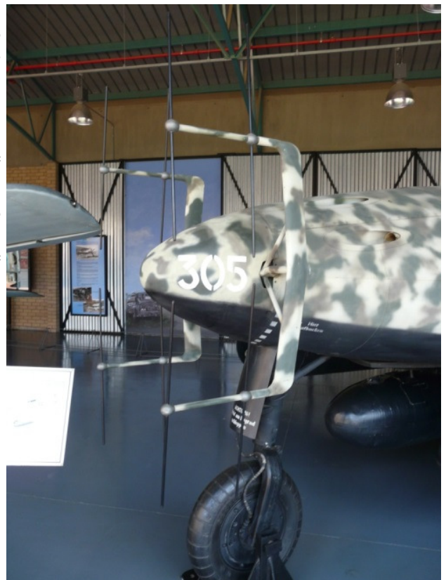
Night fighter radar antennae on the nose of the Messerschmitt 262 jet fighter in the museum of military history, Saxonwold.
