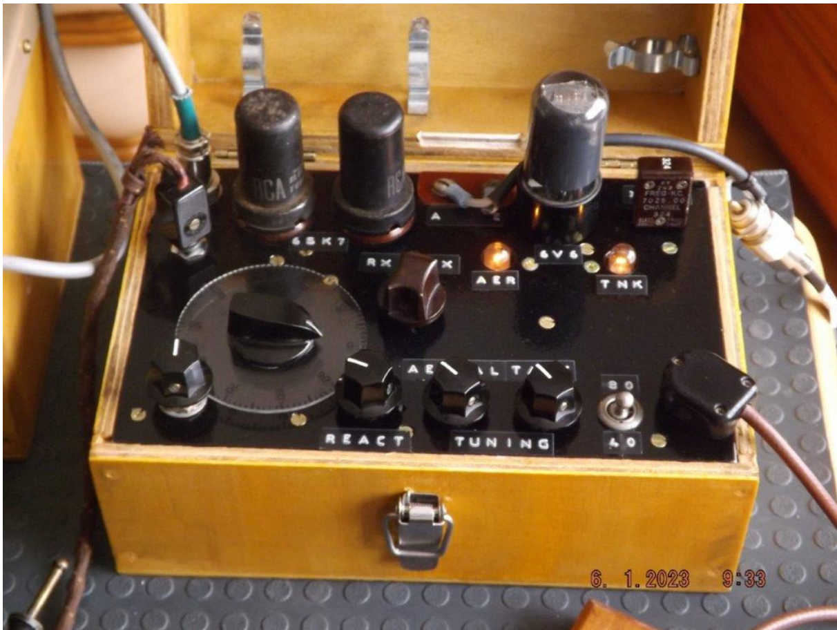
The set in action, note the Aer and Tnk indicators showing good coupling
