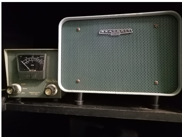
HB10B SWR Meter and SB600 Speaker
