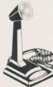
Factory wired for use with the TR7/DR7, modes: push-to-talk or VOX, dynamic, high impedance, frequency response: 300-5000 Hz, output: -48 dB at 1 kHz (0 dB = 1V/microbar), 4 pin connector.
