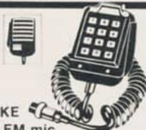
The auto-patch encoder and mic are a single unit. It features high accuracy IC tone generator, & Digitran® keyboard. Power for tone encoder from transceiver via mic cable. Encoder audio level adjustable from 1mV to 5mV with internal potentiometer. Low output impedance. 4-pin plug.
