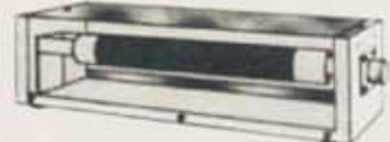
**DRAKE DL-1000** air cooled dummy load. Power rating 1000 watts, SWR 1.5:1 max. 0-30 MHz. SO-239 connectors. Expanded rating limitation when used with the Drake FA-7 cooling fan.
