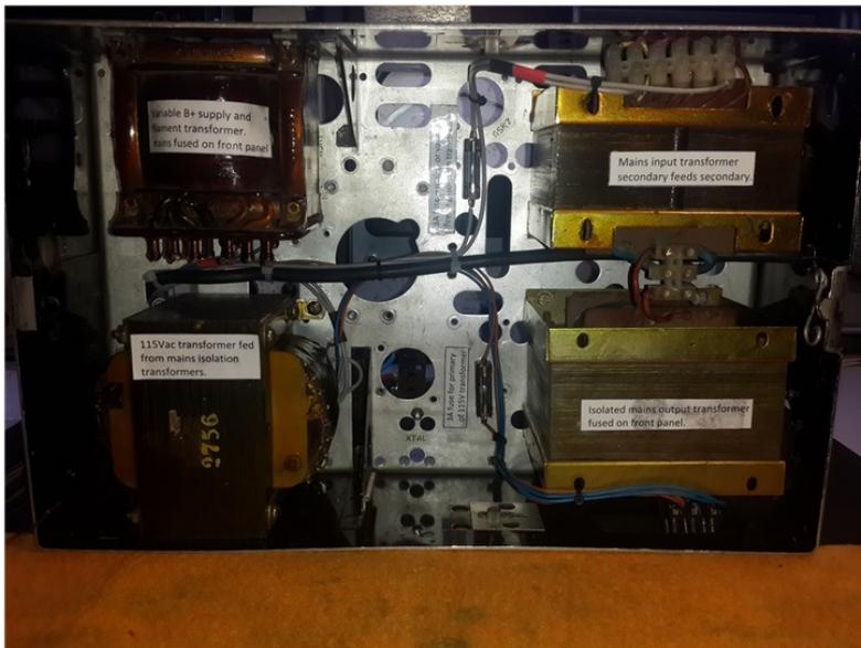
18Kg of iron neatly fit on the rear end of the enclosure.
