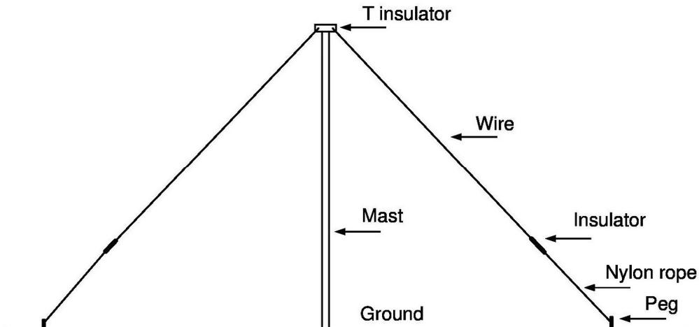
**Figure 8 Inverted typical installation**
