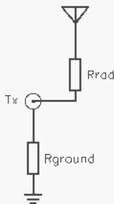
Figure 11 Vertical antenna
