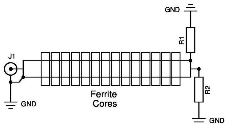
Figure 9 Test arrangement for W2DU current balun
