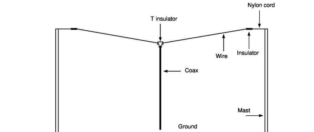
**Figure 7 Dipole diagram showing sag due to coax**
