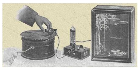
Left a turntable with electric pick up, in the middle a Loewe OE333 receiver and right a speaker type Loewe EB71 (1928)
