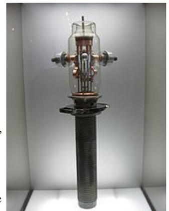
High power triode used in pre-WW2 radio transmitter, in Berlin
