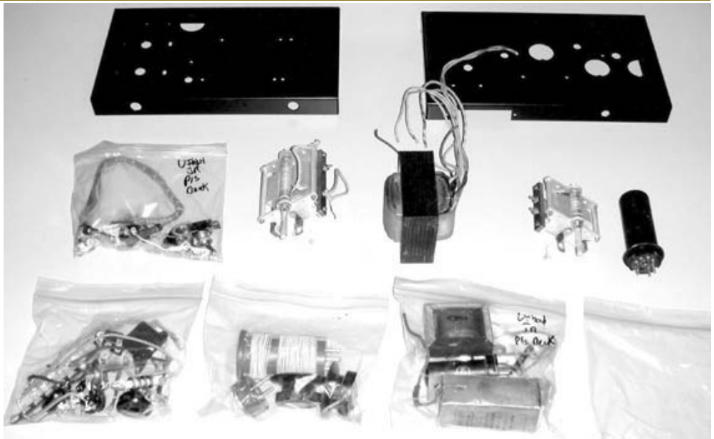
Power Supply and RF deck after disassembly
