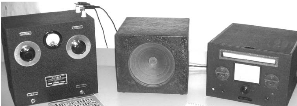
Author's National FB7/Utah Jr. station. Key and receiver power supply not transmit/receive shown.
