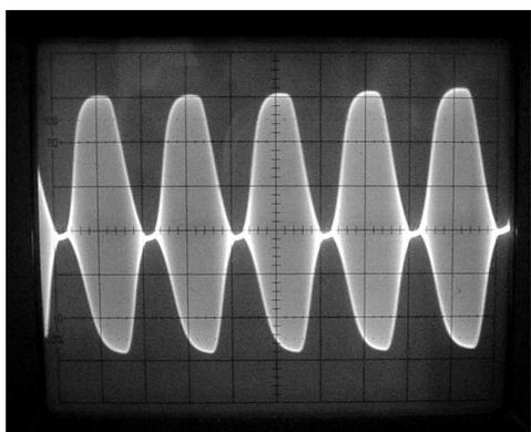
**Figure 5** **Over modulated carrier**
